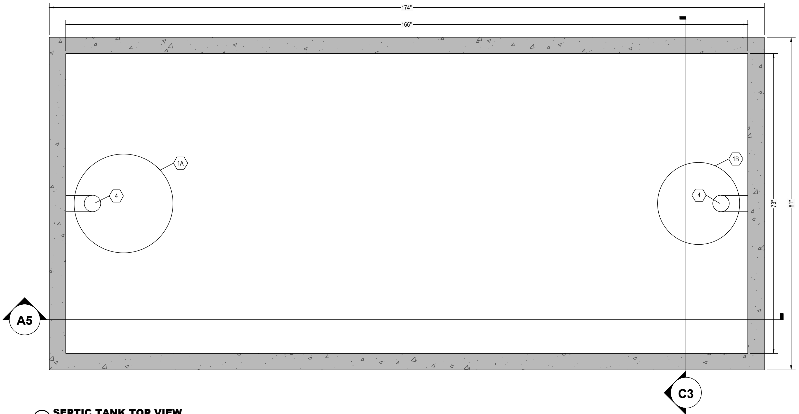
C5 SEPTIC TANK TOP VIEW 1" = 1"
